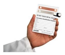
Purafil's CCC (Corrosion Classification Coupons) can be used comprehensive corrosivity report of your facility which will identify the contaminant class in the air and also the environmental classification (G1, G2, G3 or Gx) as per ISA 71.04-2013. All it takes is to expose the coupons to the Data centre and/or Control centre area for 30 days. The India partner Ripple Effect, helps the client deliver these
